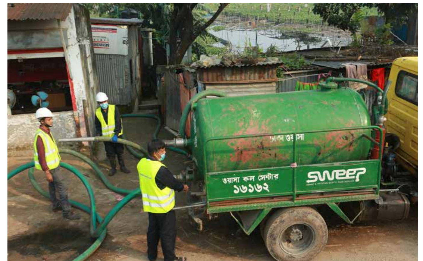
SWEET vacuum tanker in Dhaka, Bangladesh – enabling the private sector to provide fecal sludge management services – Credit: © WSUP
